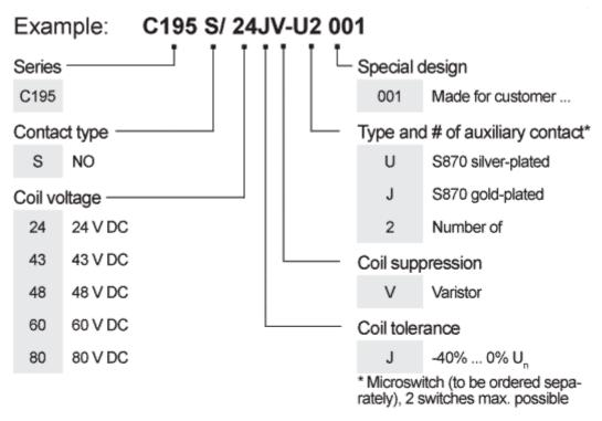
Type S contactors are DC NO contactors fitted with magnetic blowout. Here the NO contact functions as circuit-breaker with high breaking capacity in an enclosed space.
